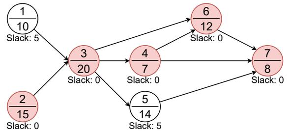
**Figure 3: The example workflow from Figure 2, with “Slack” annotations for the amount of slack identified per task using the look-ahead method (see § 2.3).**
