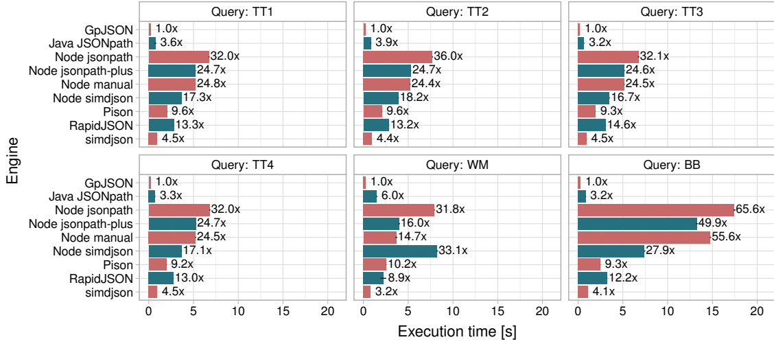
Figure 4: Comparison of GpJSON with other libraries on all queries and datasets. GpJSON is running on A100. Lower is better.
