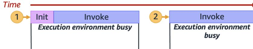
**Figure 4.4:** Sequential executions with respect to the incoming requests, when a single execution environment handles two requests one after the other. (10).
