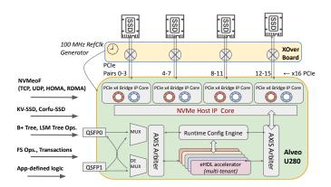
Figure 2: Schematic diagram of the Hyperion.
